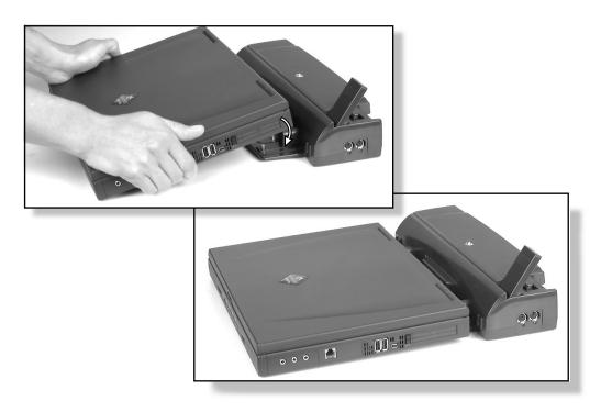
4 Press down on the release latch until it snaps into place.
