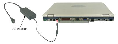
The battery starts charging as soon as you plug the power cord into an electrical outlet. The battery charges faster if the computer is turned off during charging.
