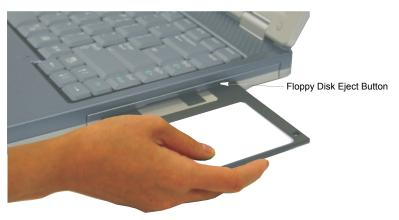
To remove a floppy disk, press the floppy disk eject button on the front of the floppy drive.
