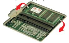
**b.** Hold the memory module by the edges and pull it forward out of the compartment.
