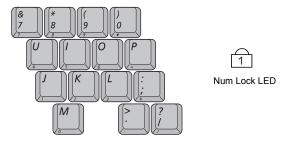
Press <Fn+F9> to turn on the embedded numeric keypad. The numeric functions of the keypad are enabled and the Num Lock LED turns on. (See "Reading the System" Status Lights" on page 22 for the location of the Num Lock LED.)
