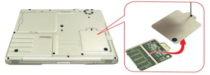
3. Grasp the edge of the door and pull the door off the chassis.
