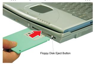
To remove a floppy disk, press the floppy disk eject button on the front of the floppy drive.
