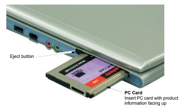
Windows automatically assigns computer resources (such as communication ports and memory addresses) to the PC Card installed in your computer.
