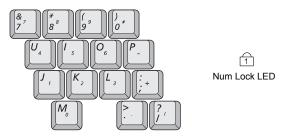
Press < Num Lock > to turn on the embedded numeric keypad. The numeric functions of the keypad are enabled and the Num Lock LED turns on. (See "Reading the System Status LEDs" on page 27 for the location of the Num Lock LED.)
