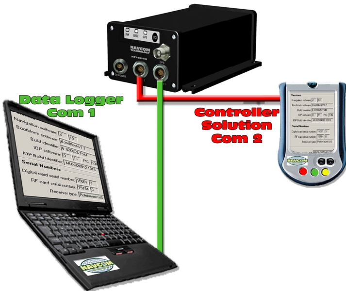
Figure 8: Communication Port Connections
