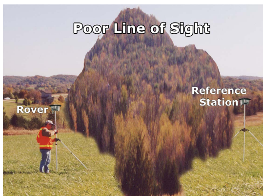
Figure 8: Poor Line of Sight RTK setup
