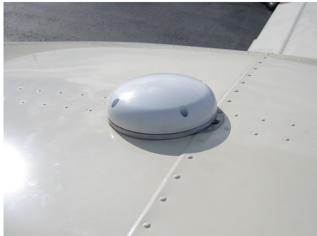
Figure 2: Antenna Mounted to fuselage
