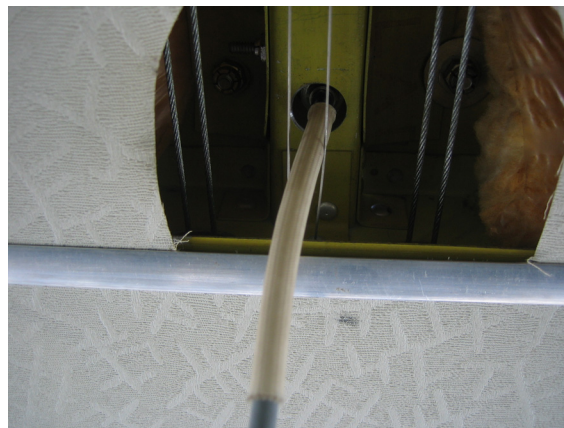
Figure 3: Antenna Cable Entering Cabin
