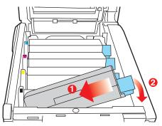
**10.** Pressing gently down on the cartridge to ensure that it is firmly seated, push the coloured lever (1) towards the
