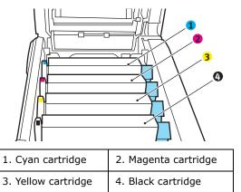
It will be necessary to remove the four image drums to gain access to the paper path.
