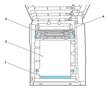
To remove a sheet just entering the fuser (3), separate
