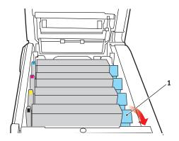
**3.** Lift the right-hand end of the cartridge and then draw the cartridge to the right to release the left-hand end as shown, and withdraw the toner cartridge out of the printer.
