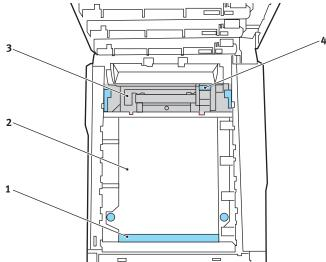
• To remove a sheet with its leading edge at the front of the belt (1), carefully lift the sheet from the belt and pull it forwards into the internal drum cavity and withdraw the sheet.
