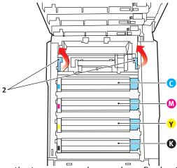
Finally, close the top cover and press down firmly at both sides so that the cover latches closed.
