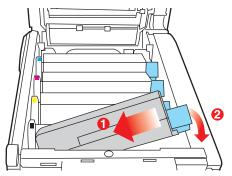
**10.** Pressing gently down on the cartridge to ensure that it is firmly seated, push the coloured lever (1) towards the rear of the printer. This will lock the cartridge into place and release toner into the image drum unit.
