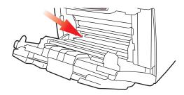
**14.** Pull out the paper tray and ensure that all paper is stacked properly, is undamaged, and that the paper guides are properly positioned against the edges of the paper stack. When satisfied, replace the tray.
