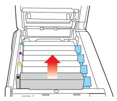
**4.** Put the cartridge down gently onto a piece of paper to prevent toner from marking your furniture and to avoid damaging the green drum surface.
