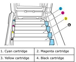
It will be necessary to remove the four image drums to gain access to the paper path.
