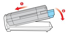
**9.** Push the coloured release lever (1) away from you to lock the toner cartridge onto the new image drum unit and release toner into it.
