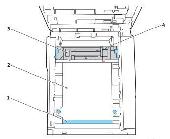
• To remove a sheet just entering the fuser (3), separate the trailing edge of the sheet from the belt, push the fuser pressure release lever (4) towards the front and down to release the fuser's grip on the sheet, and withdraw the sheet through the drum cavity area. Then allow the pressure release lever to rise again.
