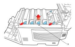
**5.** Lift the edge of the side cover slightly at the two points shown, and pull the cover away from the printer at the
