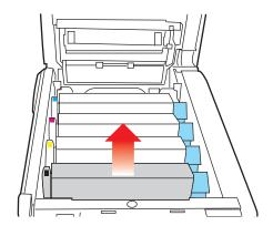
**5.** Put the cartridge down gently onto a piece of paper to prevent toner from marking your furniture and to avoid damaging the green drum surface.
