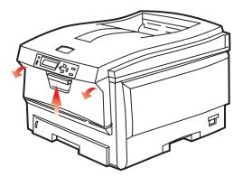
**13.** Check inside the cover for sheets in this area and remove any that you find, then close the cover.
