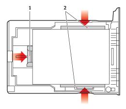
**4.** Adjust the rear stopper (1) and paper guides (2) to the size of paper being used.
