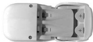
Figure: Opened charger with polarity markings
