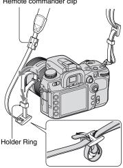
When threading the strap through the holder ring, hold the tip of the strap with your finger, and slide the holder ring rather than the tip of the strap into position to secure the strap.
