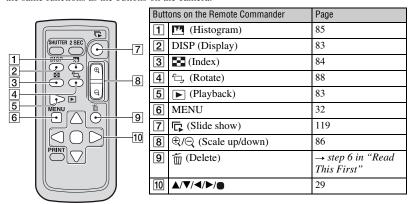
• The other buttons are used when the camera is in recording mode or is connected to a PictBridge printer (pages 60, 148).
