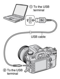
Use the fully charged battery pack or the AC Adaptor/charger (not supplied). 2 Turn on the camera and the computer, then start the "Remote Camera Control".
