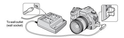
To connect the adaptor, set the POWER switch of the camera to OFF, flip open the cover, and insert the plug of the AC Adaptor/charger into the DC IN terminal.
