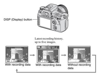
• The DISP (Display) button switches the recording data display on and off in other playback modes, such as on an enlarged screen.
