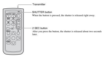
Verify that the subject is visually in focus, and point the transmitter at the remote sensor located on the front of the camera, then press the SHUTTER or 2 SEC button.
