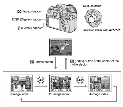
Rotating the rear dial switches the index images screen-by-screen. This is convenient when you want to switch to the next screen quickly.
