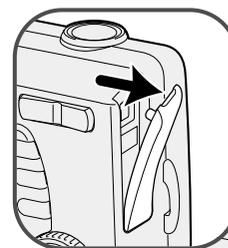
Lift the terminal cover from the top (1). The cover is attached to the body to prevent loss.
