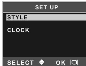
Use the scroll buttons (3) to select the style option. Press the display/enter button (4) to continue.
