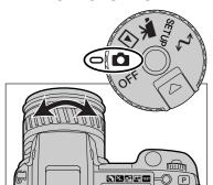
With the mode dial set to still-image recording, the camera will be on and the electronic viewfinder (EVF) and LCD monitor will activate.
