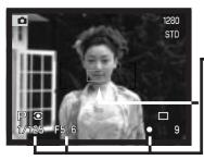
Place the subject within the focus frame. Press and hold the shutter-release button partway down or press the AF/AEL button.
