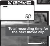
When the camera is not recording, the data-panel and monitor frame counters will show the maximum time in seconds can be recorded with the next movie clip. A maximum of 60 seconds will be displayed until the amount of remaining time falls below one minute, then the remaining number of seconds that can be recorded will be displayed.
