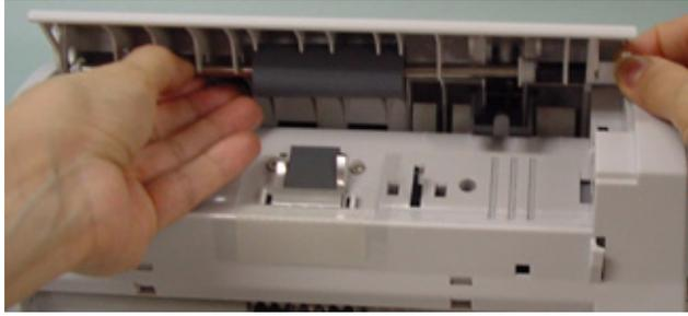
⇒The Pick roller unit is removed downwards.
