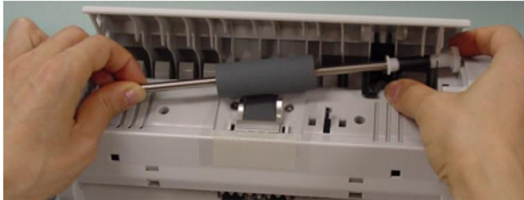
4. Attach a new Pick roller unit to the scanner.
