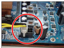
Plugged from a 4-pin ATX12V power.
