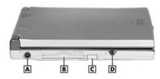
${\bf A}$  – AC power port  ${\bf B}$  – PC card slot  ${\bf C}$  – PC card eject button  ${\bf D}$  – Earphone microphone jack
