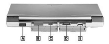
A - IR port B - Not used C - VGA port D - Serial port E - USB port
