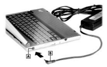
A - AC power port B - AC adapter cable
