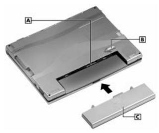
A – Battery connectors B - Battery release latch C - Lithium-lon battery pack
