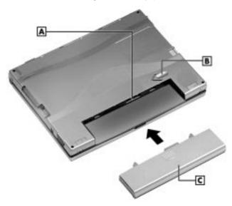
A – Battery connectors B – Battery release latch C – Lithium-Ion battery pack
