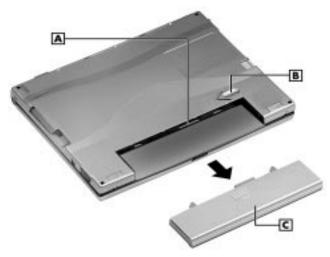
${f A}$  – Battery connectors  ${f B}$  - Battery release latch  ${f C}$  - Lithium-Ion battery pack
