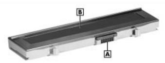
A – Battery connectors B – Lithium-Ion battery pack
