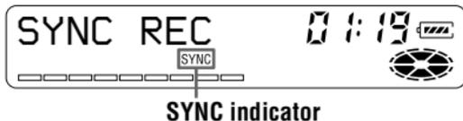
“SYNC” does not appear if optical cable is not connected to the recorder.
