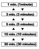
Only when using the batteries, the time for the auto power off function can be specified. When using the AC adapter (sold separately), the time for the auto power off function is fixed in 30 minutes and cannot be changed.
