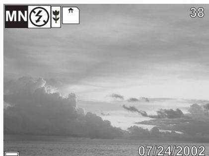
**OSD Mode:** the image and on-screen information OSD are shown on the LCD screen
