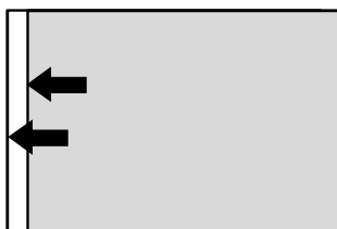
Adjust horizontal deviation by pushing the control stick to the left or to the right
