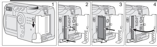
Slide the card-slot door release down to open the card-slot door (1).
