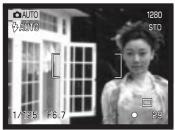
Without lifting your finger from the shutter-release button, recompose the subject within the image area. Press the shutter-release button all the way down to take the picture.
