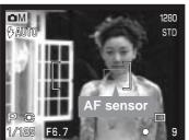
Switching between the wide focus area and the spot focus areas is simple. Press and hold the controller (1) until the wide-focus-area frame lines change to the spot-focus-area display. Press and hold the controller again to return to the wide-focus-area frame lines.
