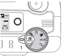
Turn the mode dial to automatic recording (1); all camera operations are now fully automatic. The autofocus, exposure, and imaging systems will work together to bring beautiful results effortlessly.
