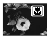
**MACRO** - used for close-up photography between 16 and 60 cm from the CCD. When the macro mode is selected, the lens will automatically zoom to the correct position. The zoom position cannot be changed. The LCD monitor will automatically activate and should be used to compose the picture. The viewfinder cannot be used because of parallax. The flash will not fire when set to an autoflash mode (p. 30).
