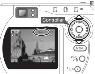
The zoom lens is operated by the controller. Pressing the down key (W) will zoom out to the wide-angle position of the lens. Pressing the up key (T) will zoom in to the telephoto position of the lens.
