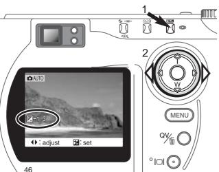
To adjust the exposure, press the exposure-compensation button (1).
