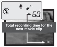
Before recording, the data-panel and monitor frame counters will show the maximum time in seconds can be recorded with the next movie clip. A maximum of 60 seconds will be displayed until the amount of remaining time falls below one minute, then the remaining number of seconds that can be recorded will be displayed.
