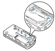
To fit the metal terminals of the battery pack and FOMA terminal, hold down the battery pack to the direction of ③, and insert in the direction of ④.
