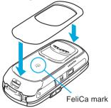
Align the FIT cover with the FeliCa mark side of the Mova and press the edge of the cover with your finger to fix it to the Mova.
