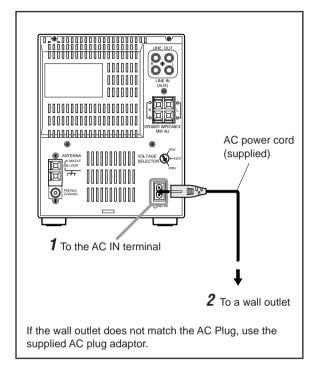
When connecting the AC power cord into a wall outlet, the unit automatically starts display demonstration.
