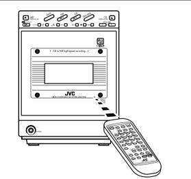
When using the remote control, point it at the remote sensor on the electronic swing panel.
