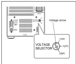
Use a screwdriver to rotate the voltage selector so the voltage number the voltage arrow is pointing at is the same as the voltage where you are plugging in the unit.
