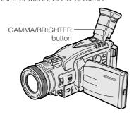
When the subject is backlit, the image will appear dark if it is recorded normally. The gamma brightness compensation function improves the picture by increasing the brightness of the subject while leaving the brighter portion of the image unaffected.
