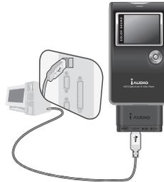
2. Connect the USB 2.0 terminal of the subpack to the PC using the USB cable provided.
