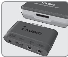
1. Connect the subpack to the bottom of the iAUDIO X5V main unit.
