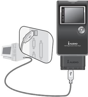
1. Connect the device to the PC using a USB cable.
