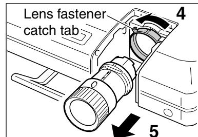
**Procedure for loosening the stiff lens fastener ring**
