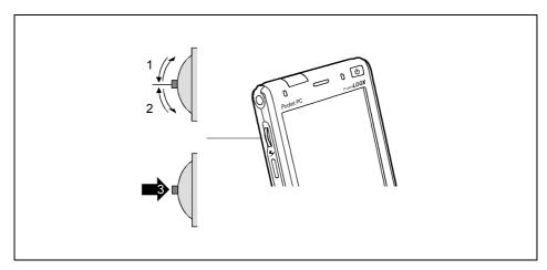
With the scroll button you can scroll up or down, forward or backward (1, 2) within the menu. You activate menu entries by pressing the scroll button in the centre position (3).
