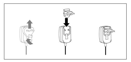
Slide the suitable mains adapter plug into the PSC11R-050 mains adapter in the direction of the arrow until it engages.
