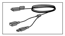
With the optional USB Host cable you can use your Pocket PC as a USB Host device and connect various USB devices, such as a MEMORYBIRD, to the Pocket PC.
