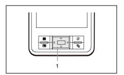
With the navigation key (1) you scroll within the menus (up, down, to the left and right) and activate menu entries by pressing the centre of the navigation key.
