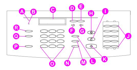
Look for the following buttons and features on the control panel. These buttons and features are used to fax paper-based documents, make copies, and adjust settings for the HP LaserJet 3100 product.
