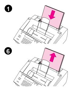
After you have cleaned the printer parts, use this procedure to print and use a cleaning page. This cleaning page may help remove toner specks on your printed pages.
