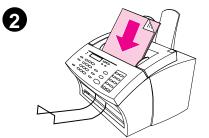
Whether you want to fax, copy, or scan, the procedure for loading the document is the same. If your document is on a regular weight paper (from 12 to 28 lb or 46 to 105 g/m²), use "To load normal items." If your document is a transparency, in a carrier sheet, or is not on regular weight paper, use "To load special items."
