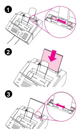
You can load up to 100 sheets of 20 lb (75 g/m²) paper into the paper input bin. The HP LaserJet 3100 product prints, copies, and prints received faxes using media from the paper input bin (or the single-sheet input slot).
