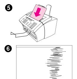
The HP LaserJet 3100 product was calibrated at the factory. However, you may need to recalibrate the scanner if you notice that sent faxes, copies, or items scanned to the computer have black or white lines running through them.
