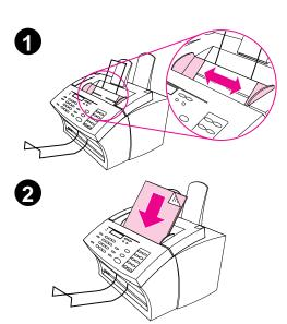
Whether you want to fax, copy, or scan, the procedure for loading the document is the same. If your document is on a regular weight paper (from 12 to 28 lb or 46 to 105 g/m²), use "To load normal items." If your document is a transparency, in a carrier sheet, or is not on regular weight paper, use "To load special items."
