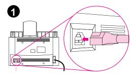
The HP LaserJet 3100 product does not have a power switch. It turns on when the power cord is connected.
