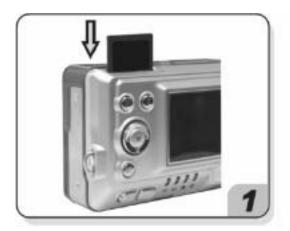
Orient the memoray card as shown, and insert it into the slot.
