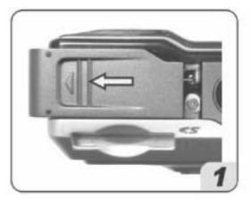
Slide the battery cover in the direction of the arrow and lift it open as shown.
