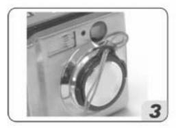
Put the lens strap through the lens strap post.
