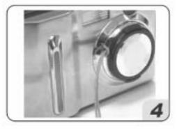
Pull the other end of the strap through the other side of the lens strap post and tighten it.
