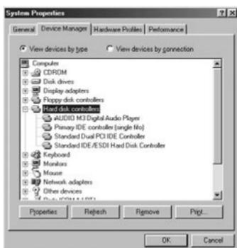
7. Finally, make sure that installation of iAUDIO M3 was completed normally by checking "iAUDIO M3 Digital Audio Player" displayed under Control Panel → System → Device Manager → Hard Disk Controller.
