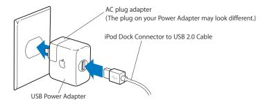
**WARNING:** Make sure the power adapter is fully assembled before plugging it into an electrical outlet.
