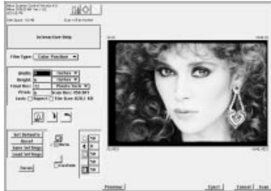
Figure 7.6 The Nikon Scanner plug-in's Main Scan dialog for monitors that display more than 832 x 624 pixels – Macintosh (Coolscan connected).
