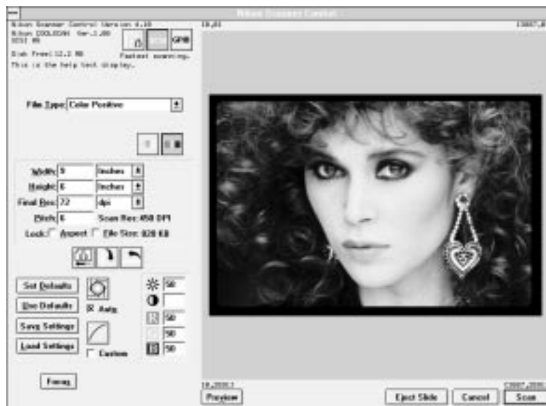
Figure 7.8 The Nikon Scanner plug-in's Main Scan dialog for monitors that have resolutions of 800 x 600 pixels or greater using small fonts, or 1024 x 768 pixels or greater using large fonts – Windows (Coolscan connected).
