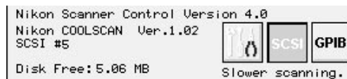
Figure 7.10b The message box (Windows) showing software version number, ROM version, SCSI ID number, and available disk space. The GPIB button is used for GPIB interfaced scanners, such as the Nikon LS-3510AF and LS-3500.
