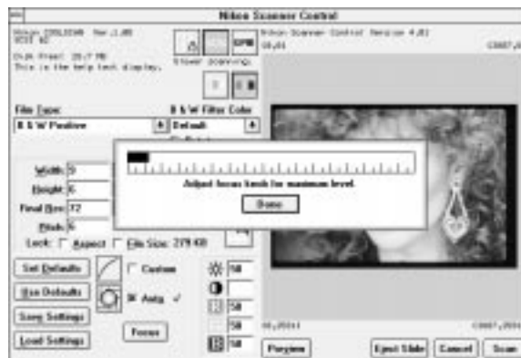
Figure 14.3b (Windows) The Scan dialog in the Metered Focus mode. The user clicks on the FOCUS button. The cursor is then placed in the preview window and clicked on the area to be focused on. A meter bar is displayed allowing the user to adjust the focus until the maximum level is indicated.
