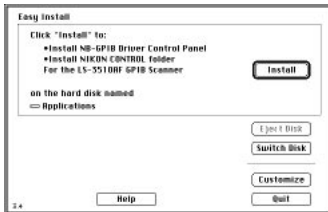
Figure 2.3 The Nikon Installer dialog for selecting Easy Install of LS-3510AF GPIB model. Click CUSTOMIZE for installation for other Nikon devices.
