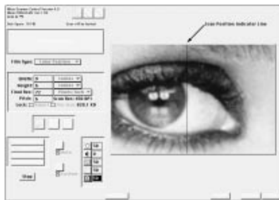
Figure 14.4a The Scan dialog in Visual Focus mode – Macintosh. The user clicks on the FOCUS button, then positions the magnifying cursor over the region of interest and clicks. The film is repetitively scanned with a highly magnified scan and displayed in the preview window, allowing the user to fine focus.
