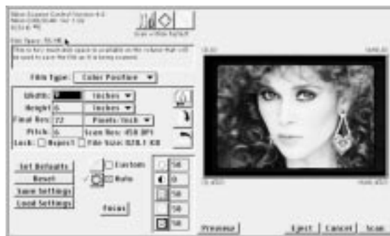
Figure 7.7 The Nikon Scanner plug-in's Scan dialog for monitors that display less than 832 x 624 pixels – Macintosh (Coolscan connected).
