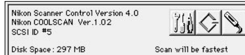
Figure 7.10a The message box (Macintosh) showing software version number, ROM version, SCSI ID number, and available disk space. The far-right button is used for GPIB interfaced scanners, such as the Nikon LS-3510AF and LS-3500.
