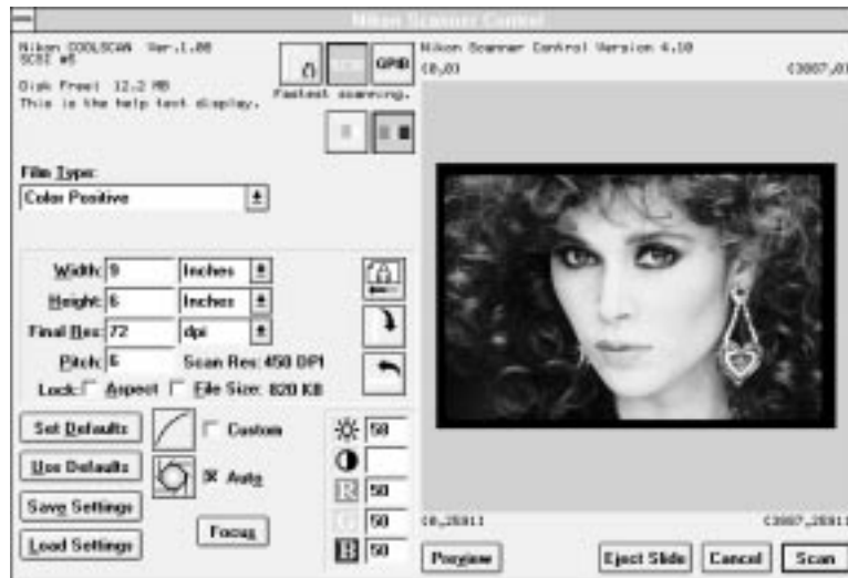
Figure 7.9 The Nikon Scanner plug-in's Main Scan dialog for monitors that have resolutions of 640 x 480 pixels, using small fonts, or 800 x 600 pixels using large fonts – Windows (Coolscan connected).
