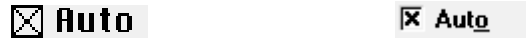
Figure 13.4 AUTO check box with no Autoexposure check mark indicates an autoexposure will occur before the next scan – Macintosh and Windows.
