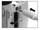
Connect the video cable plug to the VIDEO IN terminal on the TV.
