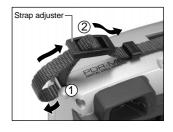
Pass the leading end through the fastener and pull tight.
