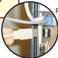
Plug the other end of the USB connector into an available USB port on your computer.
